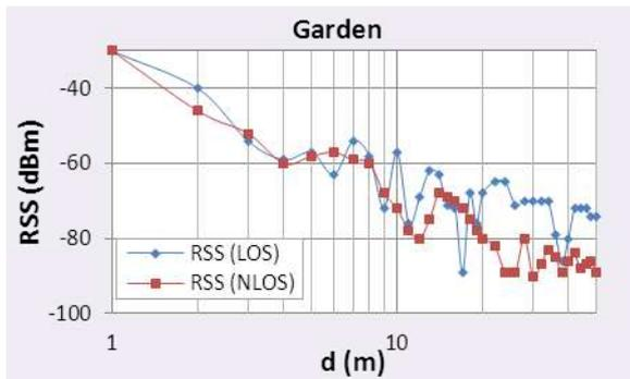
Fig.5. RSS with (a)LoS and (b)NLoS.
