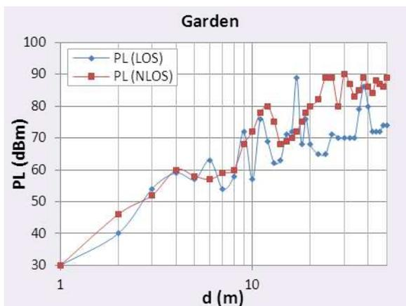
Fig.6. PL with (a)LoS and (b)NLoS.
