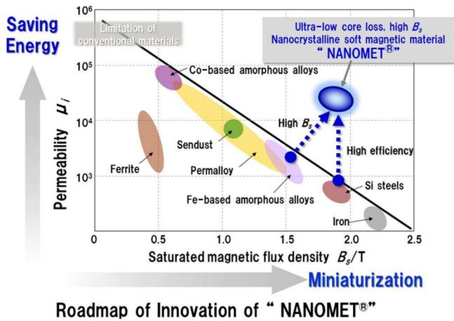
Fig. 1. Development road map of ultra low loss nanocrystalline alloy "NANOMET®"[6].
