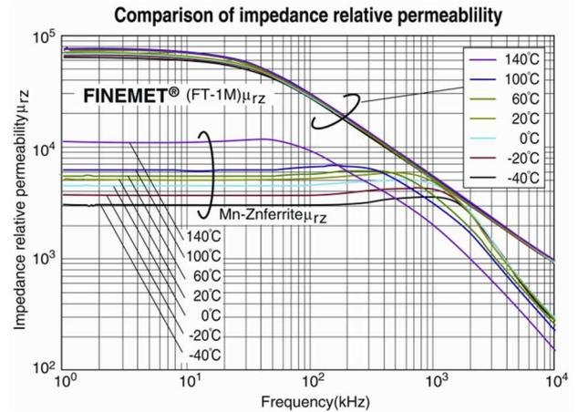
Fig. 3. Relative permeability  $\mu_r$  versus operating frequency of nanocrystalline material FINEMET and Mn-Zn ferrites [3].
