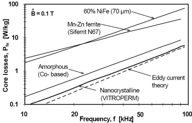
Fig. 5. Specific core losses of magnetic materials under sine wave, [7],[8].
