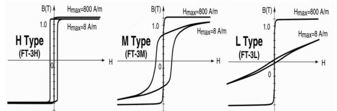
Fig. 4. Typical B-H loops for FINEMET [3].
