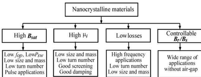
Fig. 6. Features and proper applications of nanocrystalline materials.
