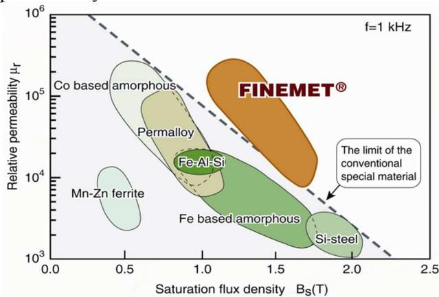
Fig. 2. Initial permeability versus saturation induction for soft magnetic materials [3].
